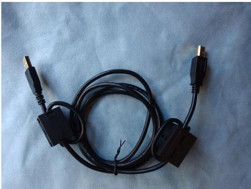
Wavenode supplied USB cable with 3-turn ferrite cores at each end.
